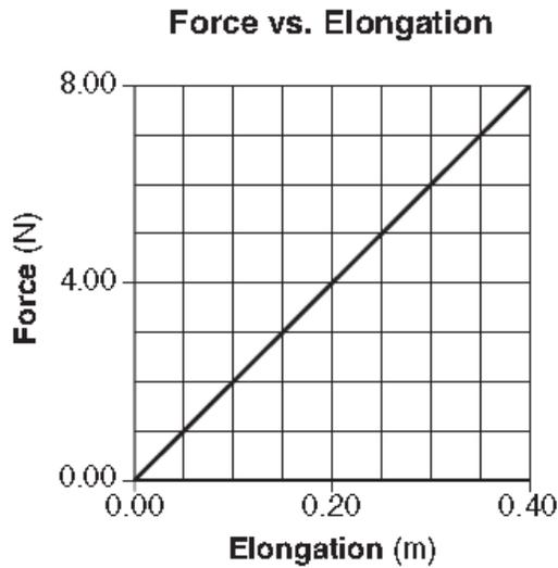
A student produced various elongations of a spring by applying a series of forces to the spring. The graph represents the relationship between the applied force and the elongation of the spring.
