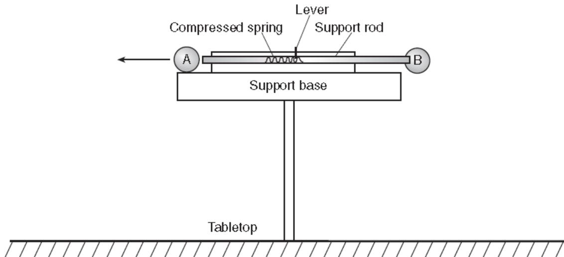
When the lever is released, the support rod withdraws from ball B, allowing it to fall. At the same instant, the rod contacts ball A, propelling it horizontally to the left.
